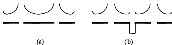
Fig. 4. Odd-mode charge distribution in the three-conductor line (a) and a pair of two-conductor lines (b). Because the charge distributions on both sets of lines are nearly identical, the pair of lines in (b) adequately models those in (a).
